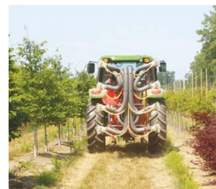
ARS's new automated spraying system can detect the presence, size, shape and foliage density of trees and then apply the optimum amount of pesticide in real time.
