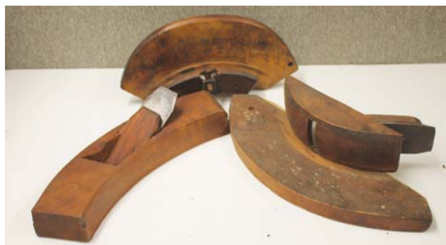
Grouping of coopering tools from the 19th century. Tight barrel croze (top); leveler (left) and a howel for tight barrel.
