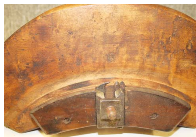
The barrel croze is used to groove the ends of the staves.
