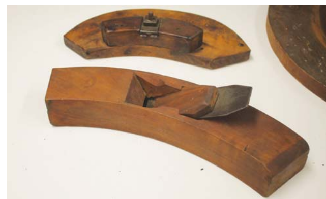
This item is described as a Leveler in the D.R. Barton & Co's Standard. The company and date that is burned into the top is D. Barton - 1832 - Rochester, NY.
